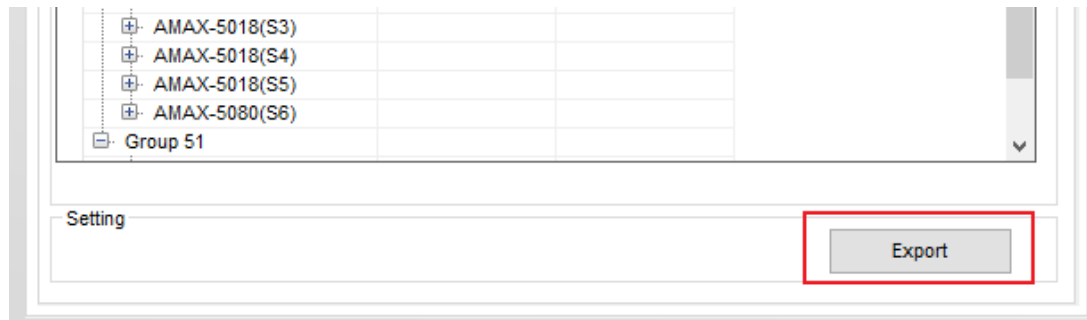
Figure 3.26 Export the ModBus TCP Address in Fixed Mode
